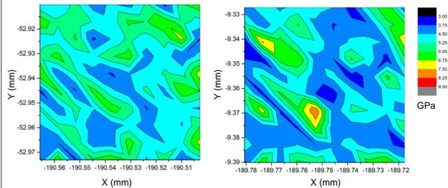
Hardness maps of HT2 (L) and HT1 (R) material, quarter section; data recorded with 3000 µm load and third loading segment. In both cases product results in islands of the hard phase separated by a sea of ferrite due to diffusivity time.
