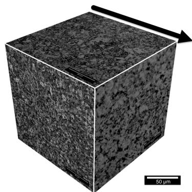
Rolling direction indicated with the arrow. Scale bars on each face represent 50 µm. Grains showed minor variability in shape and orientation on different faces.
