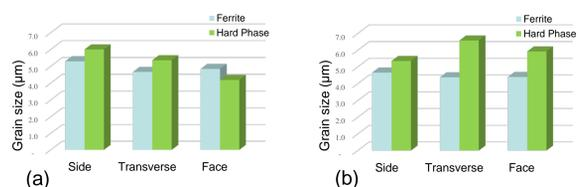
HT1 (a) and HT2 (b) grain sizes from quarter section. Grains were not determined to be shallow compared to their observed surface area. 95% confidence intervals ranged from 0.76 µm to 1.16 µm for ferrite and 1.18 µm to 1.82 µm for harder phases.
