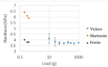
As the applied load of Vickers hardness increased, readings approached the measured hardness of ferrite obtained from nanoindentation. Vickers loads of 10g have high variation, suggesting the measurement of multiple phases. Data taken from uncoated edge sample.
