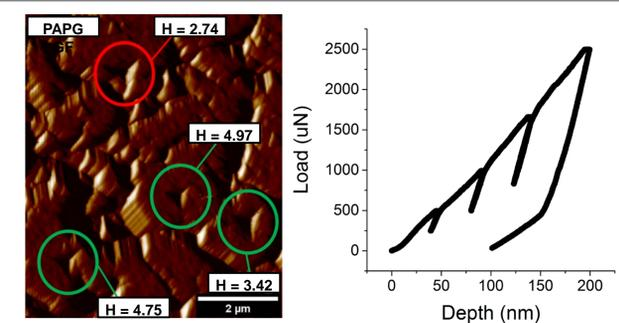
Image from the scanning probe on the Hysitron. The lower three samples, highlighted in green, are indicative of usable placements on ferrite. The indentation at the top was placed too close to a grain boundary. A sample load-depth curve is shown to the right.
