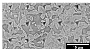
In this SEM image, ferrite can be seen as the darker phase and the lighter phase represents the harder phase. Indents can be observed within grain boundaries.
