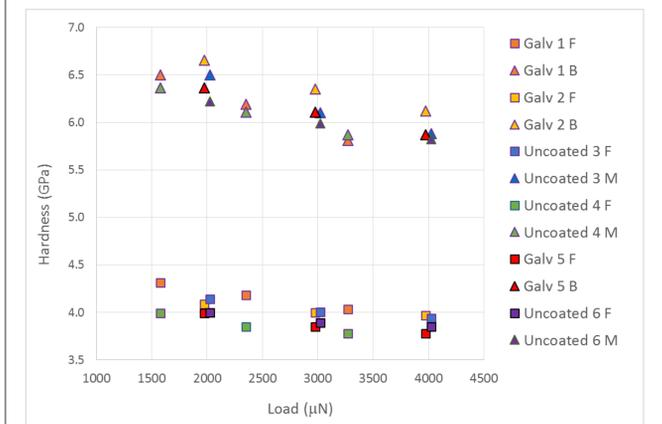
Displayed hardness values for hard and soft phases are based on average measurements from accepted indentations from the grid sampling method.
